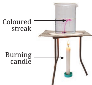
Fig. 7.5(b): Demonstration of convection in heated water
