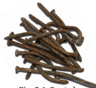
Fig. 5.4: Rusted iron nails
