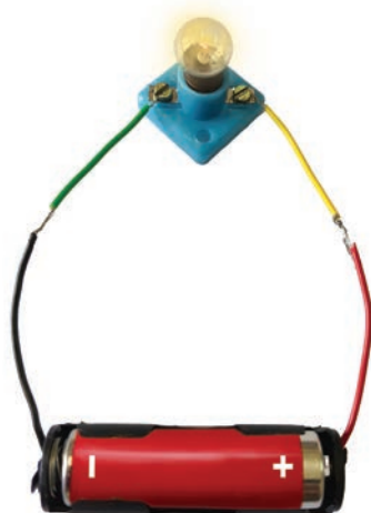
Fig. 3.9: An electrical circuit
