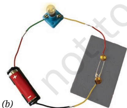
Fig. 3.12: An electrical circuit with a switch in (a) 'OFF' position (b) 'ON' position
