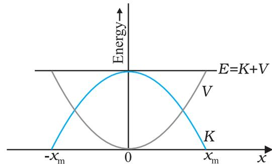
**Fig. 6.8** Parabolic plots of the potential energy  $V$  and kinetic energy  $K$  of a block attached to a spring obeying Hooke's law. The two plots are complementary, one decreasing as the other increases. The total mechanical energy  $E = K + V$  remains constant.
