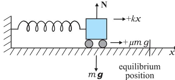
**Fig. 6.9** The forces acting on the car.
