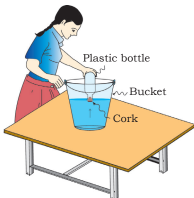
Fig.9.10.3 Arrangement to show the existence of buoyant force
